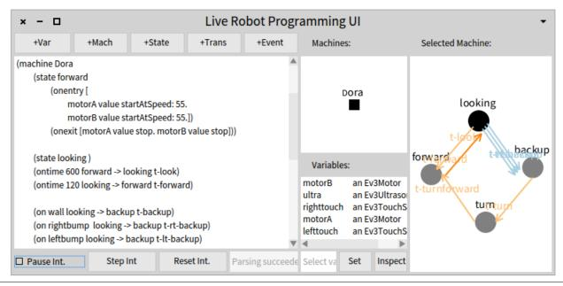
Figure 2. The LRP editor showing part of the example of this text: the Dora machine.
