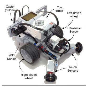
**Figure 1.** The Lego Mindstorms robot of the explorer behavior example.
