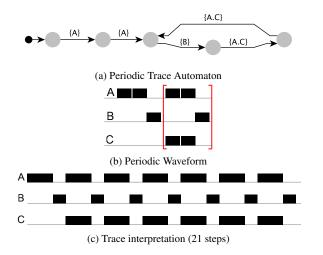
Figure 2: Cyclic simulation trace and different visualisations with CLOCKSystem for the SDF example in Fig 1
