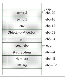
**Figure 2.** Bee Stack frame layout for Object>>#foo:bar: in memory on x86
