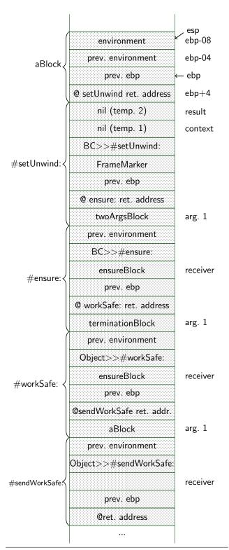
Figure 4. Stack frame layout after aBlock activation
